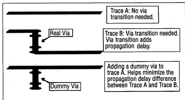
**Figure 9**—Example of adding a "dummy" via to a trace
