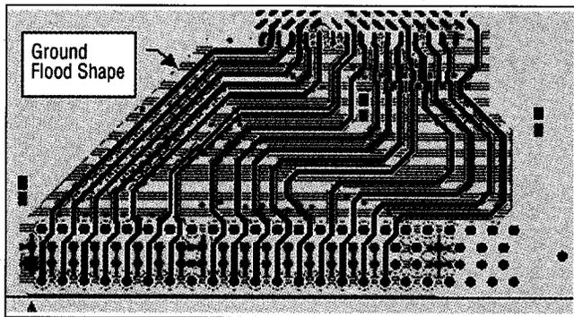
**Figure 10**—Routed RDRAM channel with ground flood shape
