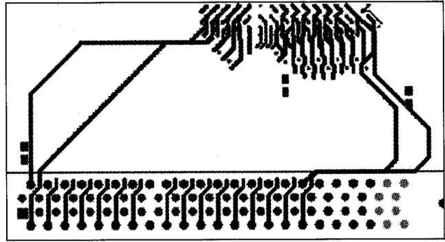
**Figure 7**—Lines expanded to match longest routed length
