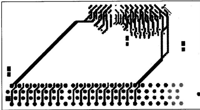
**Figure 6**—Routing outside lines before length-matching to longest line
