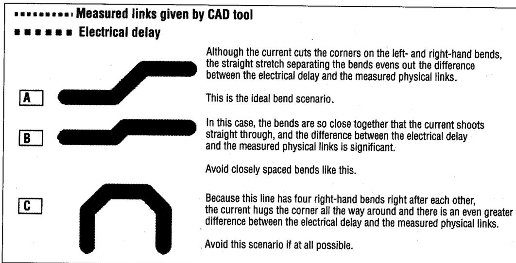
**Figure 3**—Example of current cutting the corner on bends
